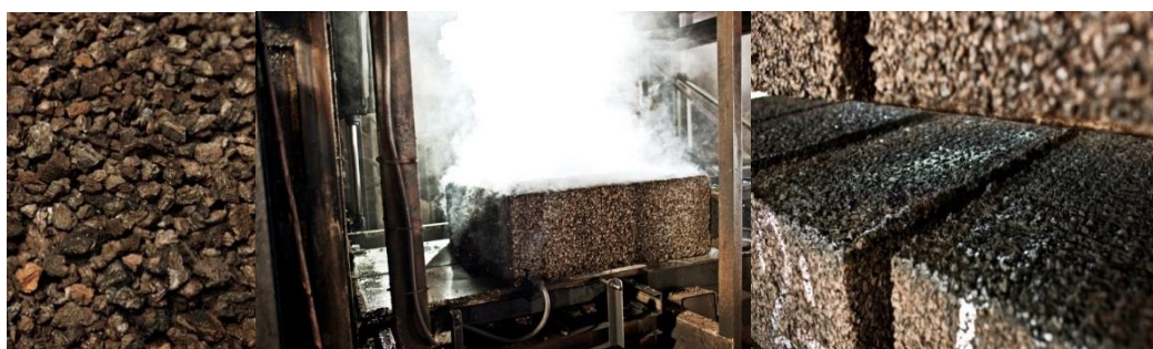
Figure 21. The Expanded Cork Board is made by expanding cork grains through the action of steam. It is agglutinated from resins in the cork itself, without the use of any synthetic agents.
