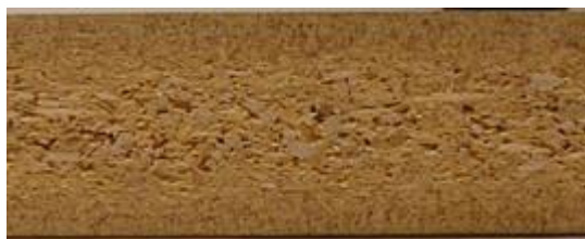
Figure 11. Cross section of particleboard
